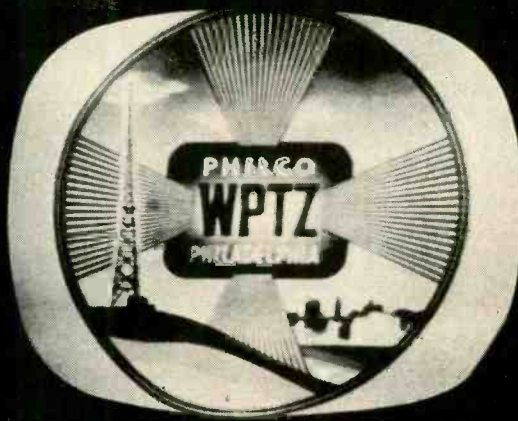
Appearance of screen when cosine yoke is used without the corrector magnets.
